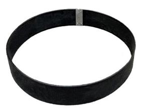
These simple and cost-effective tree protectors are made from 12mm recycled plastic sheeting, and can be supplied in any size to suit the job at hand. The examples illustrated are 730mm diameter by 200mm high, and sit 100mm into the surface for secure fixing.
